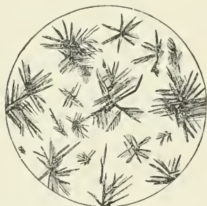
Stellate Crystals obtained by heating Corrosive Sublimate, magnified 30 diameters.
